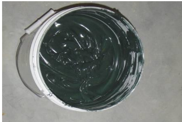
Picture #16: Fully mixed sealant
