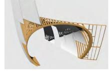
The Radius Track Design Team used Rhino 3D modeling software to design the 218 unique pairs of steel stud and track panels for the framing of the hull's exterior surface.
