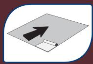
Place the Transguard® 4000 roll on the concrete floor, fiber side down, and unroll the blanket in a straight line.
