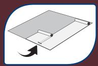
After the first layer has been rolled out, roll out the next layer of Transguard® 4000.
