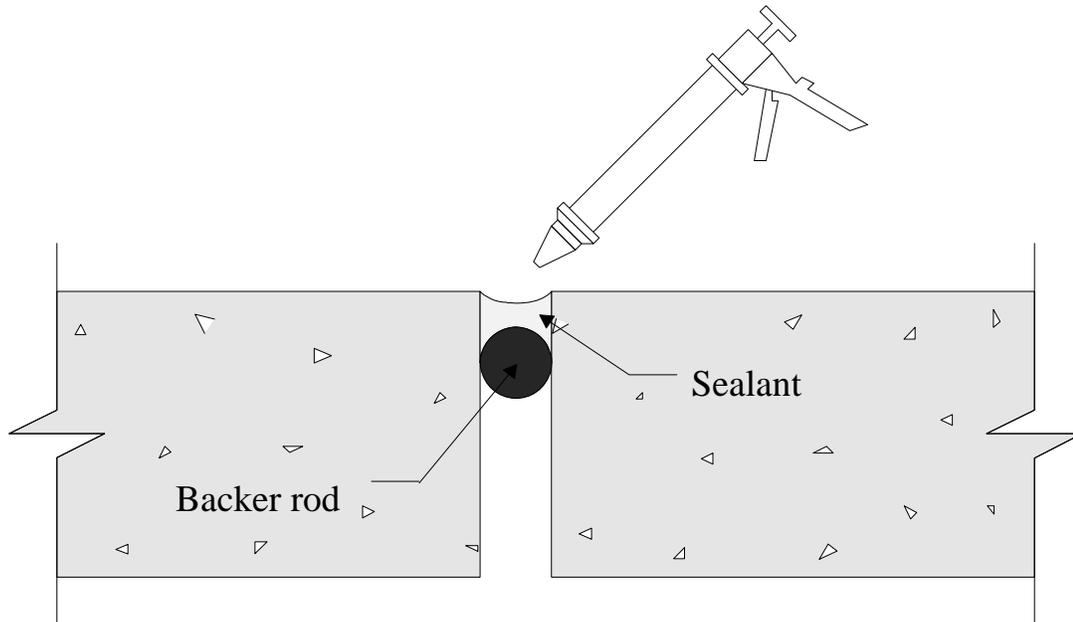
1. Install appropriate backer material to prevent three-sided adhesion and to control sealant depth.
