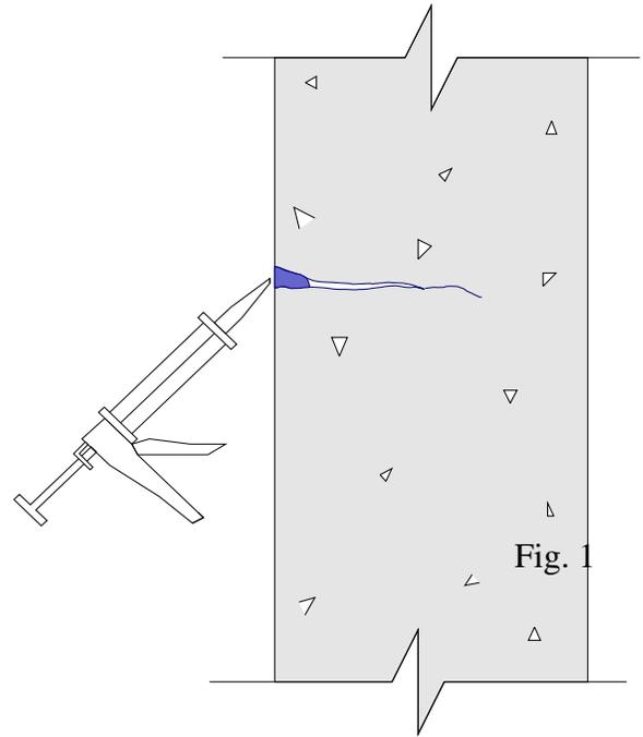
Figure 2 - Notch & Seal
