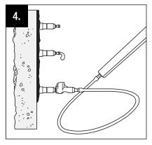
5. Go to the last port where epoxy appeared while injecting the first port, open it, and continue injection at this port. If the epoxy has set up and the port is bonded closed, move to the next clean port and repeat the process until every portion of the crack has refused epoxy.
