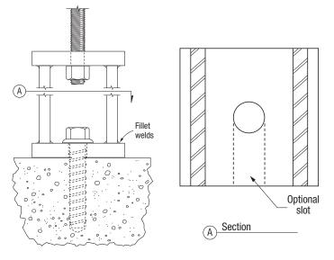
**Note:** Torque-testing of anchors is not considered to be a suitable method of verifying anchor tension capacity since the torque-to-tension relationship of concrete anchors varies depending on installation and base material conditions.
