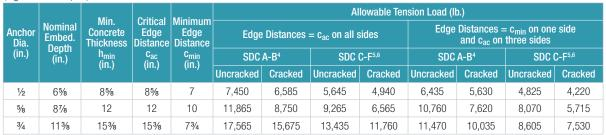
1. Allowable tension loads are calculated based on the strength design provision of ACI 318-11 Appendix D using a conversion factor of  $\alpha = \frac{1}{2}$ . The conversion factor  $\alpha$  is based on the load combination assuming 100% seismic load.
