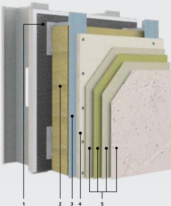
1. **Water-Resistive Barrier** – Sto AirSeal® provides a single source, seamless and fully integrated layer for air and weather tightness.
