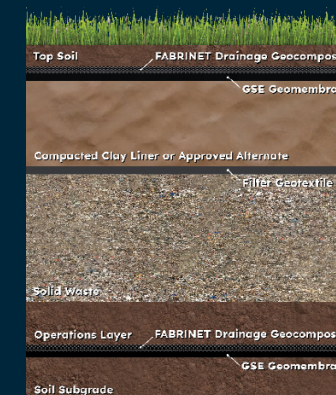
Municipal Waste Landfill with Geosynthetics
