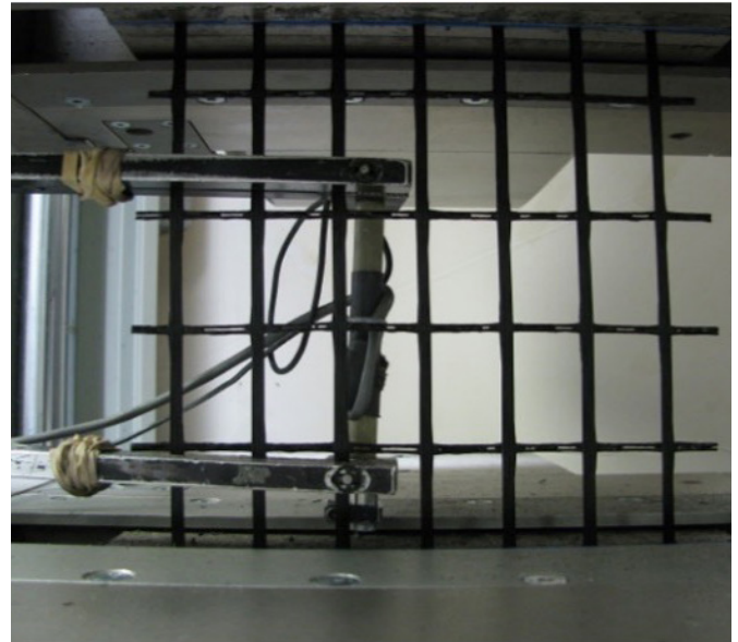
Figure 2: Wide Width Tensile Test of MIRAGRID
