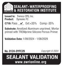
Dymonic FC is fast-curing with a skin time of 60 minutes and a tack-free time of 3 to 4 hours. This significantly reduces dirt attraction and improves the overall asthetic look. Additionally, Dymonic FC will not green crack due to early movement. The low-modulus nature of Dymonic FC allows it to provide exceptional movement capability of ± 35%.
