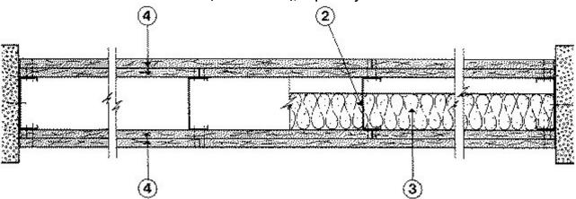
1. **Floor and Ceiling Runner** — (Not Shown) — Min. 25 MSG galv steel, 1 in. return legs, 2-1/2 in. deep (min), attached to floor and ceiling with fasteners 24 in. OC max.
