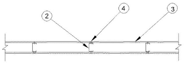
1. Framing Members\* — Floor and Ceiling Runners — (Not Shown) — For a 1 hour rating, use with Items 3, through 3K only, proprietary channel shaped, min. 3-5/8 in. wide, fabricated from min. 0.0150 in. (min bare metal thickness) galvanized steel, attached to floor and ceiling with fasteners 24 in. OC max. For a 2 hour rating, use with Items 3A through 3F, proprietary channel shaped, min.
