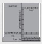
On bathroom floors, start by placing full tiles in front of bathtub or shower and along the adjoining wall to avoid cut tiles in this highly visible area.
