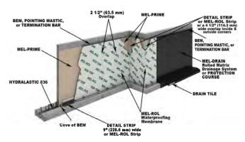
Inspect and Repair ... A thorough inspection should be made before covering and all necessary repairs made immediately. Tears and inadequate overlaps should be covered with MEL-ROL ... slit fish mouths and patch. Seal edges of all patches with POINTING MASTIC. Where applicable, horizontal applications can be floodtested for 24 hours. All leaks should be marked and repaired when membrane dries.
